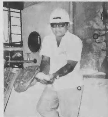
At left, Benny Kock shows the sand-like clay that goes into the clay filters for improving the Milli Pore Color quality of jet fuel. At right, Eddy Tjin Kon Fat has two handfuls of real rock salt which is used to remove water from the kerosene jet fuel.
